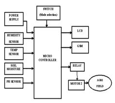
Fig. 1 Block diagram of the Proposed System
