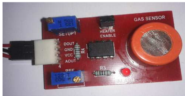
Fig. 1 Design of LPG leakage detection
