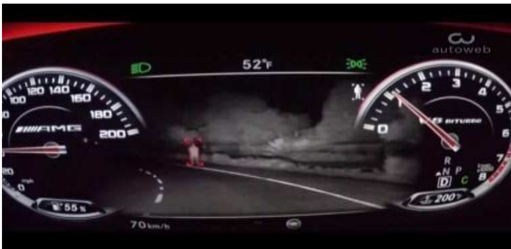
Fig. 2. Pedestrian highlighted by red mark as seen on display unit .
