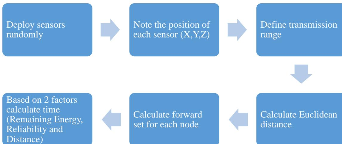
Fig. 1 Flow chart of proposed algorithm
