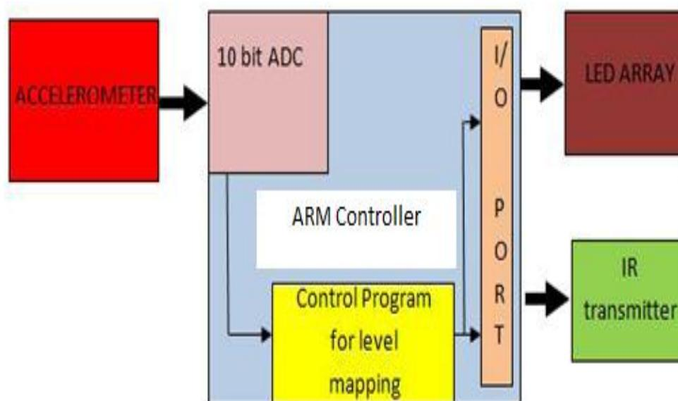
Fig. 2 Accident warning system
