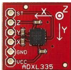
Fig. 5 ADXL335 Accelerometer
