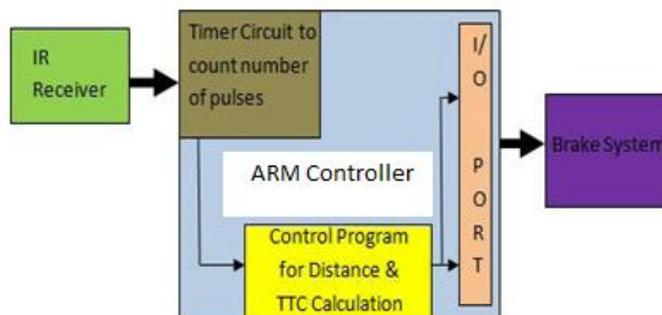
Fig. 6 Accident Avoidance System
