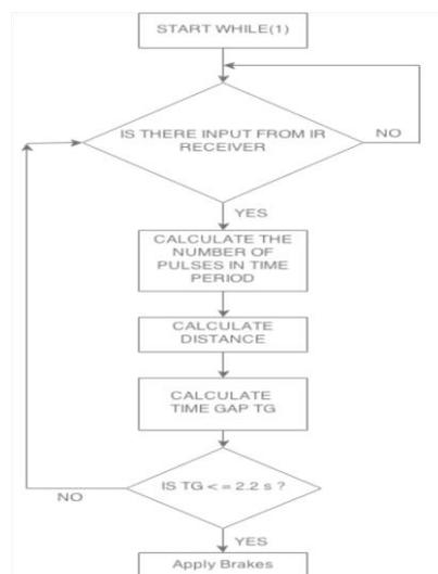
Fig. 7 Flow chart of accident avoidance system
