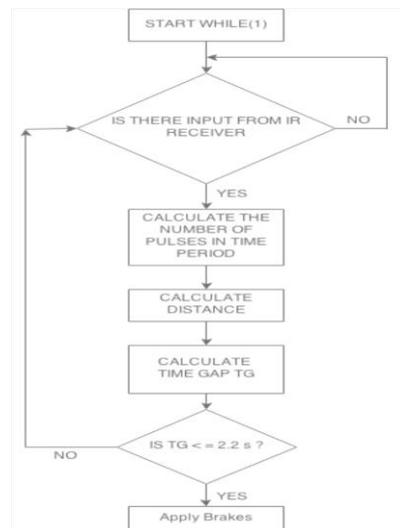
Fig. 7 Flow chart of accident avoidance system
