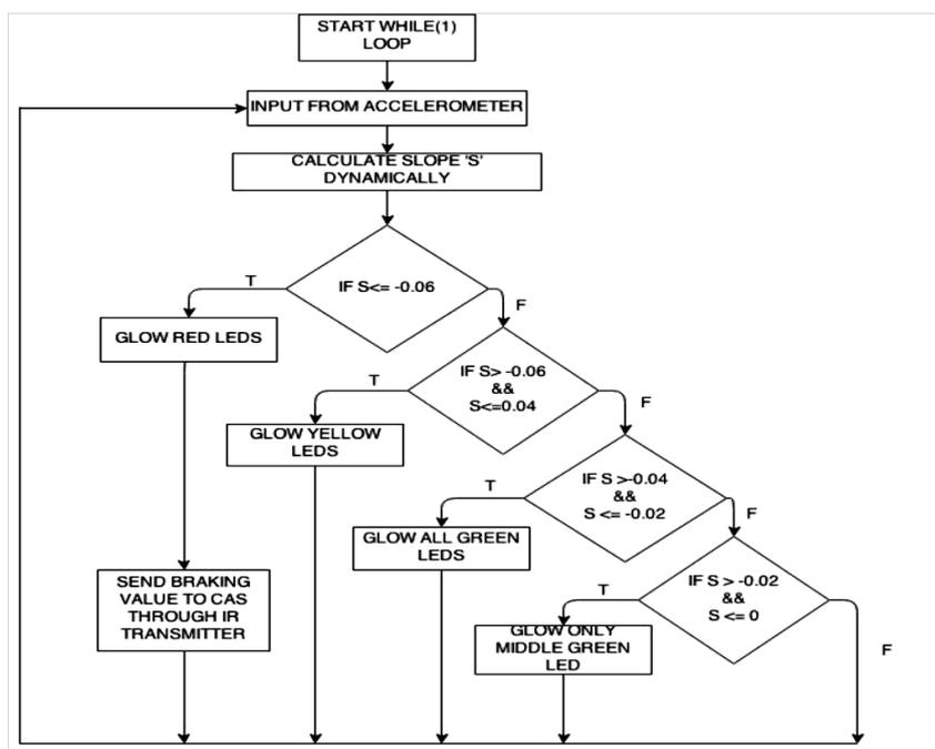
Fig. 3 Accident warning system's control algorithm
