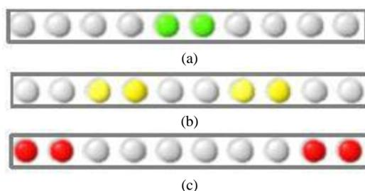
Fig. 4 (a) low breaking level shown by Green LEDs. (b) Medium breaking level shown by Yellow LEDs (c) Sudden breaking shown by Red LEDs.
