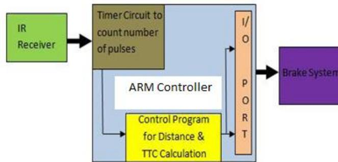
Fig. 6 Accident Avoidance System
