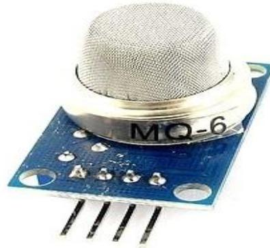
Fig. 3 MQ-6 Gas sensor
