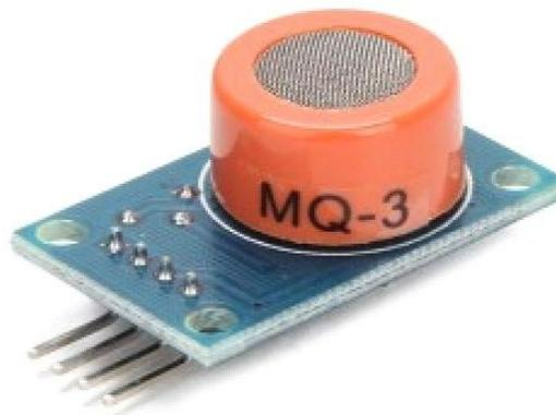
Fig. 2 MQ-3 Alcohol sensor
