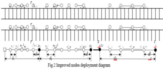
In this above figure black node is denoted as sensor node and whit node is denoted as relay node and rectangle represents the sink node. Let the Nth is sensor node, all sensor nodes are in the first row.
