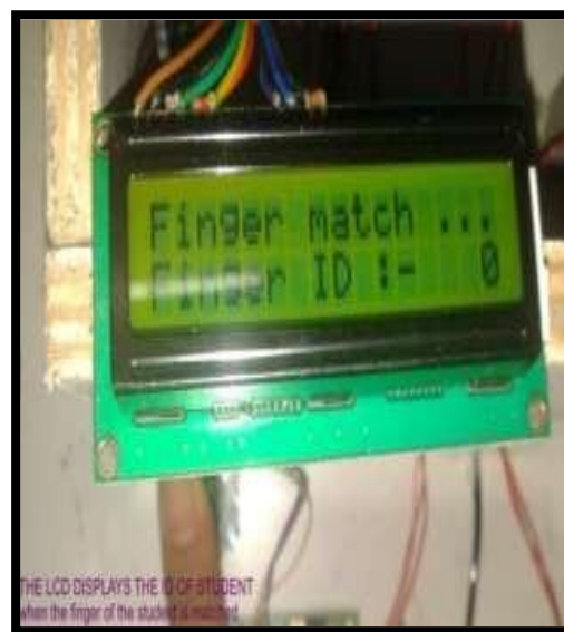
Fig. 9 (a) Automatic Attendance using Thumb Detector
