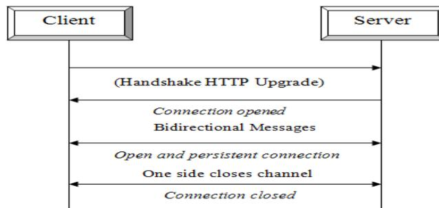
Fig.5 Web Socket connection
