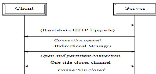
Fig.5 Web Socket connection
