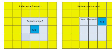
Fig.6 Reference frame (I), search area (P), current macro-block (MB)
